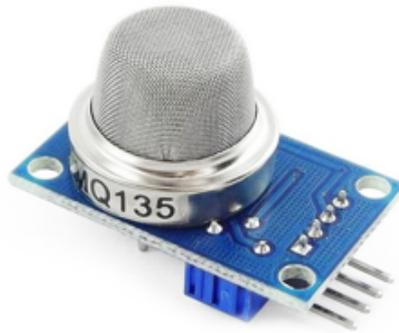
Figura 20 – Sensor de gases MQ-135.
