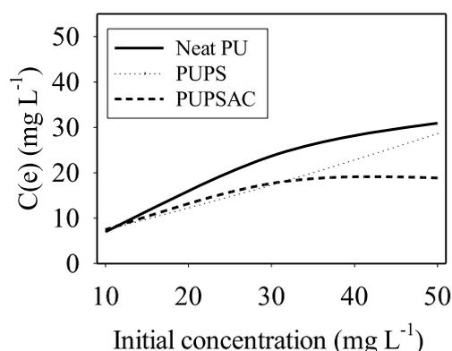
Fig. 3 - Effect of initial solution concentration on equilibrium concentration of Cr(III) from solution using PUF; 200 rpm; room temperature (25 °C); mass concentration 0.3 g L<sup>-1</sup>; pH 6.5.
