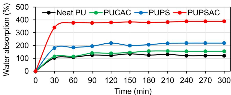
**Fig. 1.** Water absorption by PUFs. Neat Polyurethane, PUPS (Polyurethane Peach Stone), PUPSAC (Polyurethane Peach Stone Activated Carbon) and PUCAC (Polyurethane Commercial Activated Carbon).
