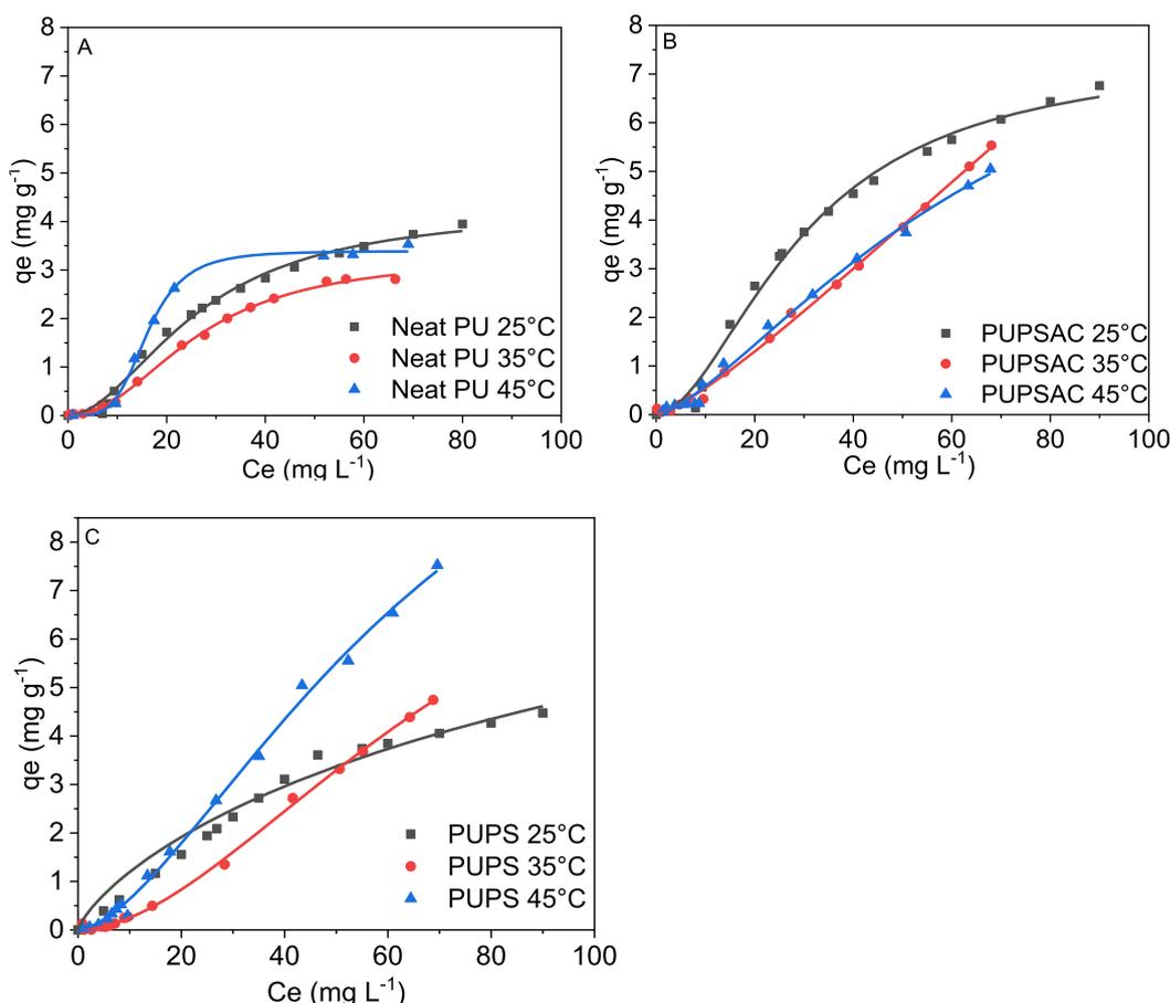
Fig. 5 – Adsorption isotherms of Cr(III) onto (A) Neat PU, (B) PUPSAC, and PUPS (between 25 and 45 °C). Mass concentration was  $1.2 \text{ g L}^{-1}$ ; and pH of the solution was adjusted to pH 6.5. The continuous line is a plot of Sips model.
