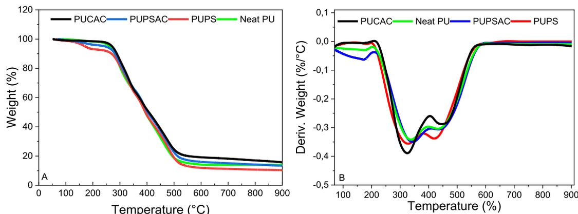
**Fig. 3** - TG (A) and DTG (B) curves of the PUF (Neat PU (Neat Polyurethane), PUPS (Polyurethane Peach Stone), PUPSAC (Polyurethane Peach Stone Activated Carbon), PUCAC (Polyurethane Commercial Activated Carbon).
