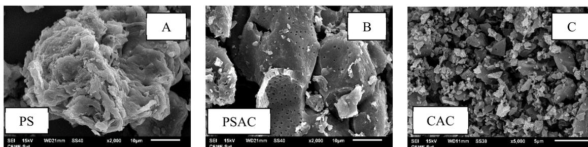
**Fig. 1** – SEM images of the fillers. PS (Peach Stone in natura) (A), PSAC (Peach Stone Activated Carbon) (B), CAC (Commercial Activated Carbon) (C).
