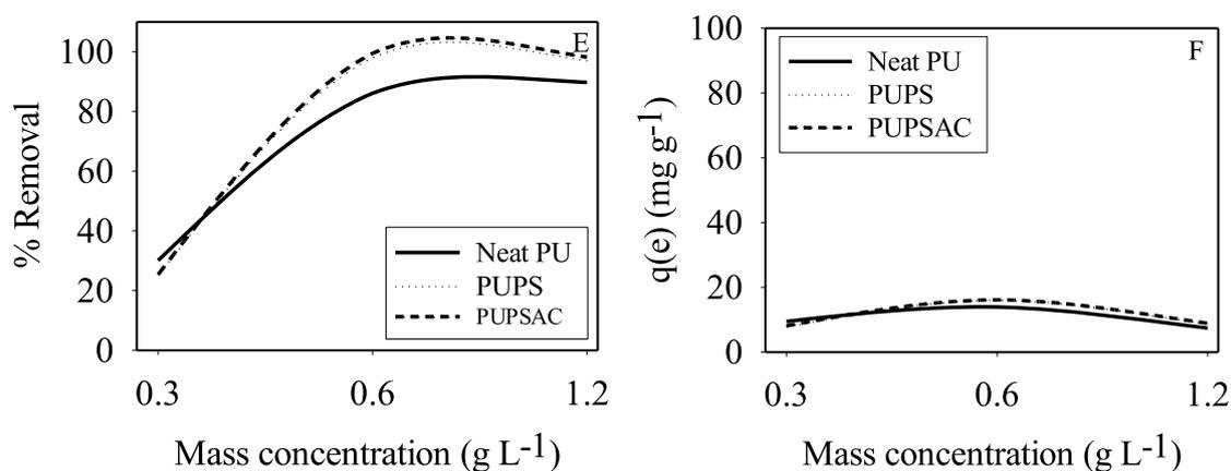
Fig. 2 - Effect of mass concentration on the removal of Cr(III) from solution using PUF;  $C_o = 50 \text{ mg L}^{-1}$  (Cr III) (A and B);  $C_o = 30 \text{ mg L}^{-1}$  (Cr III) (C and D);  $C_o = 10 \text{ mg L}^{-1}$  (Cr III) (E and F); pH 6.5; 200 rpm and 25 °C.
