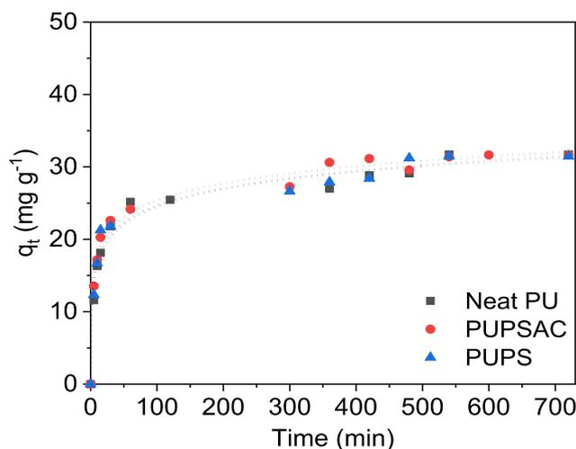
Fig. 4 – Kinetic adsorption curves for Cr(III) onto Neat PU, PUPS and PUPSAC. Experimental conditions:  $C_0$  of  $50 \text{ mg L}^{-1}$ ;  $0.6 \text{ g L}^{-1}$  of adsorbent,  $\text{pH} = 6.5$ , and temperature of  $25 \text{ }^\circ\text{C}$ . The dot line is a plot representing the Elovich fitting.
