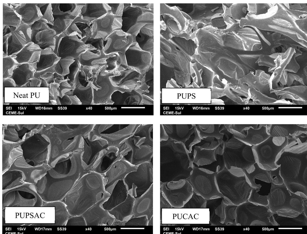
**Fig. 4** – SEM of the studied PUF. (Neat PU (Neat Polyurethane), PUPS (Polyurethane Peach Stone), PUPSAC (Polyurethane Peach Stone Activated Carbon), PUCAC (Polyurethane Commercial Activated Carbon)).
