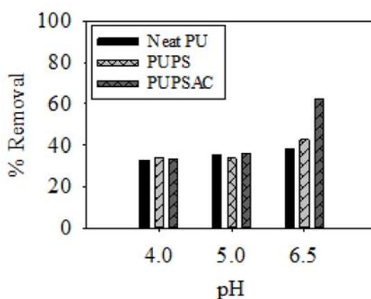
Fig. 1 - Effect of pH on the removal of Cr(III) from solution using PUF; initial concentration  $50 \text{ mg L}^{-1}$  (Cr III); mass concentration  $0.3 \text{ g L}^{-1}$ ; 200 rpm and  $25 \text{ }^\circ\text{C}$  .
