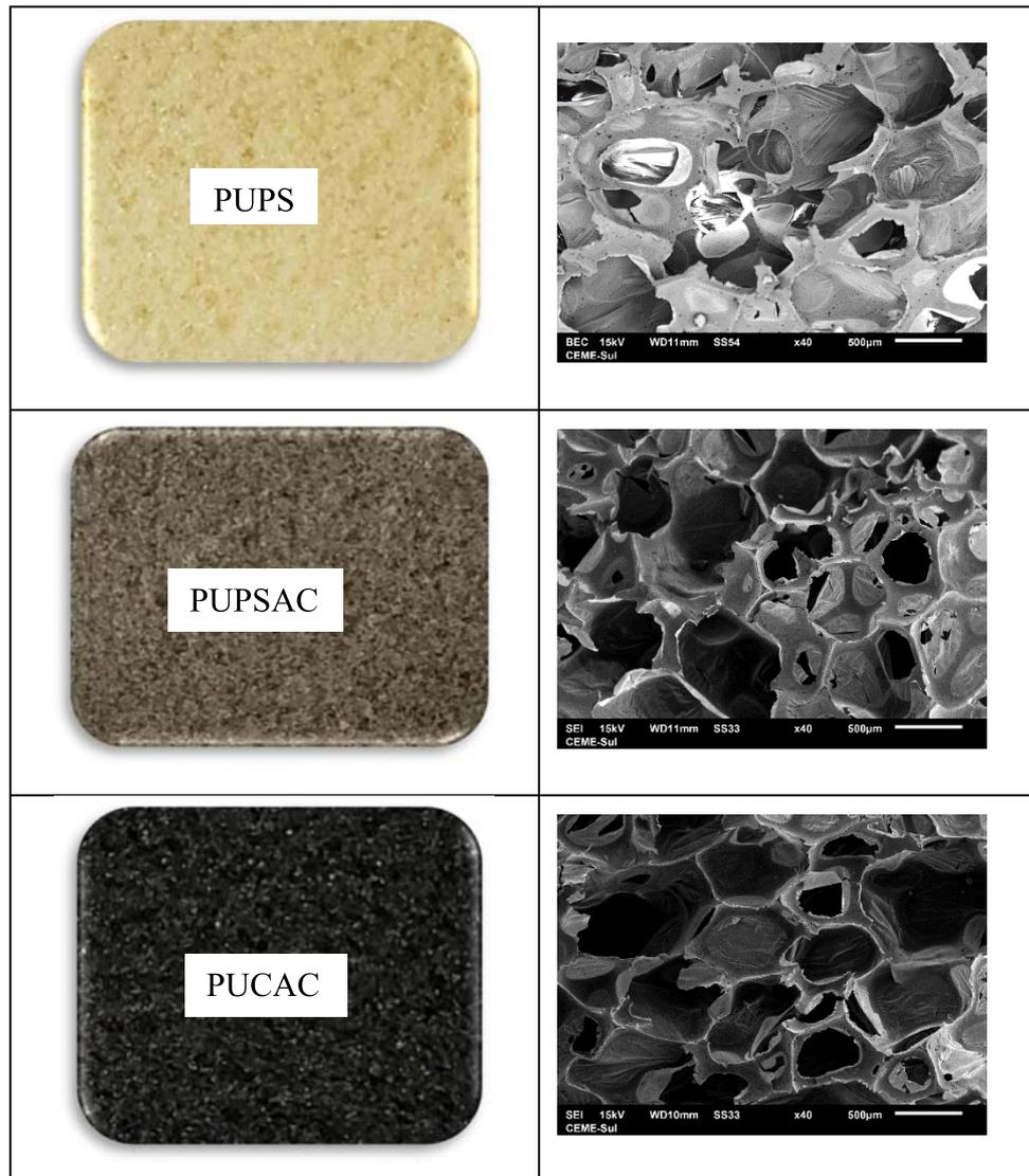
**Fig. 2.** SEM images of the studied PUFs. Neat Polyurethane, PUPS (Polyurethane Peach Stone), PUPSAC (Polyurethane Peach Stone Activated Carbon) and PUCAC (Polyurethane Commercial Activated Carbon).
