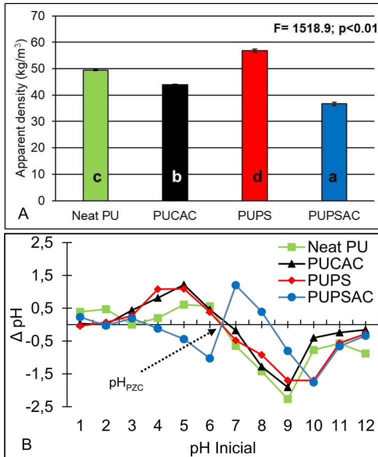
**Fig. 5** – Apparent density of the PUF (A) and Point of zero charge of the studied PUF (B); (Neat PU (Neat Polyurethane), PUPS (Polyurethane Peach Stone), PUPSAC (Polyurethane Peach Stone Activated Carbon), PUCAC (Polyurethane Commercial Activated Carbon)).
