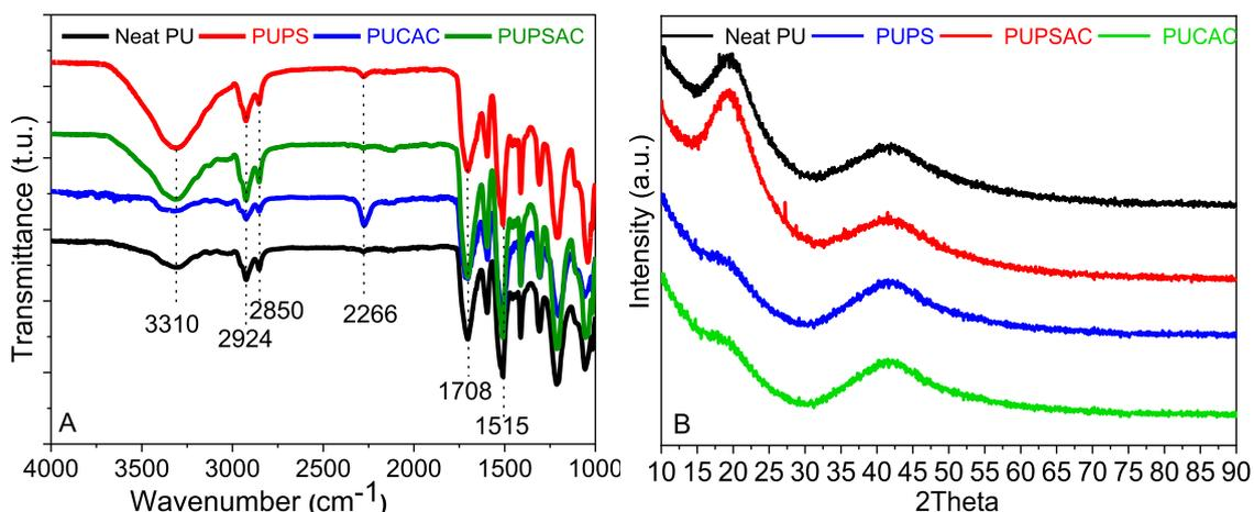
**Fig. 2** - FTIR spectra of the studied PUF (a) and X-ray diffractograms of the PUF (b); Neat PU (Neat Polyurethane), PUPS (Polyurethane Peach Stone), PUPSAC (Polyurethane Peach Stone Activated Carbon), PUCAC (Polyurethane Commercial Activated Carbon).
