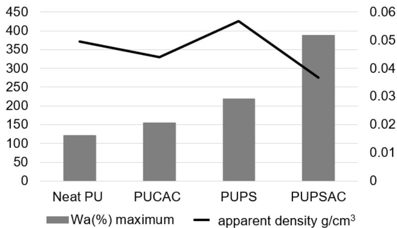
**Fig. 3.** Apparent density and maximum water absorption capacity of the PUFs
