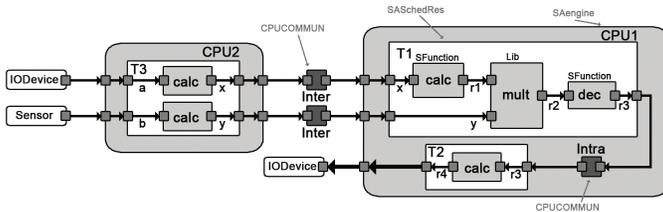
**Figure 12.** Simulink components created by setIO rule (links connecting T2 to IODevice)
