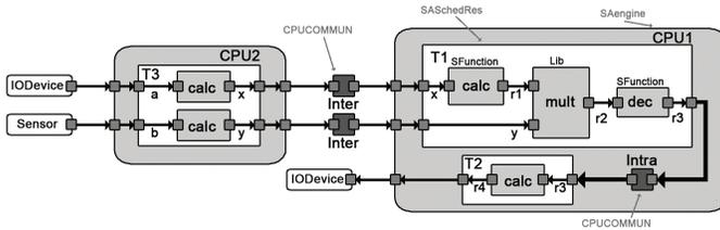
**Figure 11.** Simulink components created by IntraC rule (links connecting T1, Intra, and T2)
