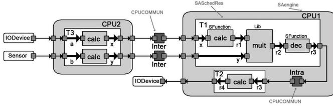
**Figure 14.** Simulink components created by rules with priority 2 (links inside threads)
