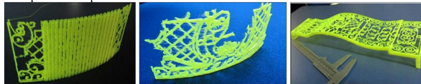
Fig. 7. Problems faced in 3D printing the balcony [8].
