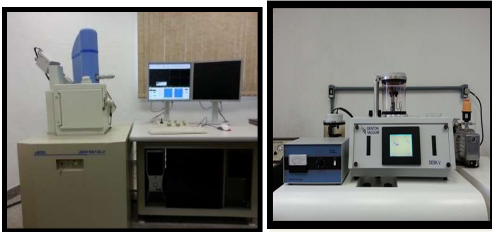
Figure 5 – Scanning electron microscopy (SEM). SEM machine (JSM 5600LV, Jeol, Japan) with a secondary electron detector (SE) SEM Images (50x, 200x, 400x, 1000X)
