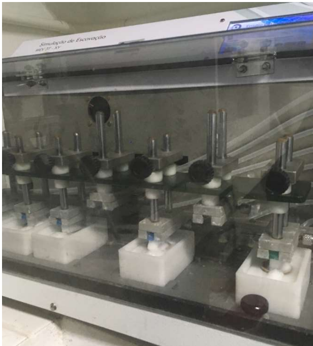
Figure 7 – Brushing machine (MEV 3Y-XT; Odeme, Luzerna, SC, Brazil)
