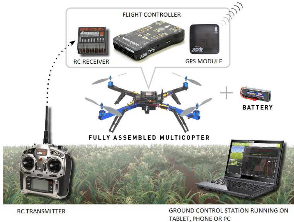
Figure 2 – Fully assembled multicopter along with its components: Ground Control Station, RC transmitter/receiver, GPS module, battery, and flight controller.
