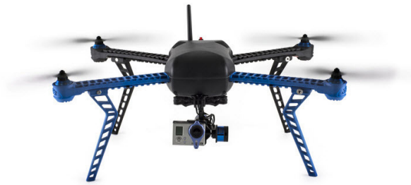
Figure 47 – IRIS quadcopter with a GoPro camera mounted on a Gimbal stabilizer.
