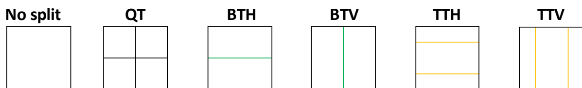
Figure 3 – Partition types of the QTMT partitioning structure.
