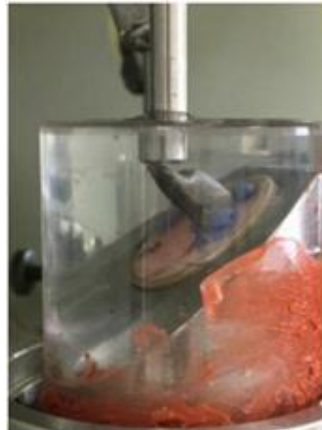
Figure 3: Specimens immersed in water at \pm 37^{\circ}\text{C} under edge to edge load
