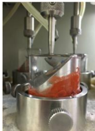
Figure 2: Specimens immersed in water at \pm 37^{\circ} C under cingule load
