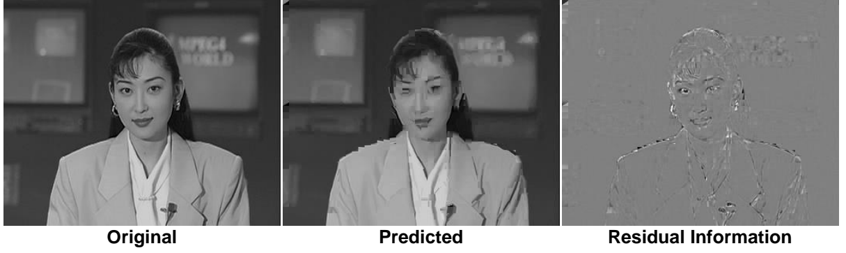
Figure 5 Left: Luminance frame of the test sequence Akiyo (Property of Stadium Inc.). Middle: Same frame predicted with 8x8 AV1 intra prediction modes. Right: Residual information obtained.
